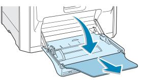
2 Load labels only in the Multi-purpose Tray with the print side down and the top, short edge in first. Adjust the guide to fit the width of the labels.
